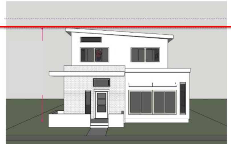
Low- Sloped Roof: 3/12 pitch or less
