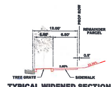
TYPICAL WIDENED SECTION WITH MIN TREE WELL
