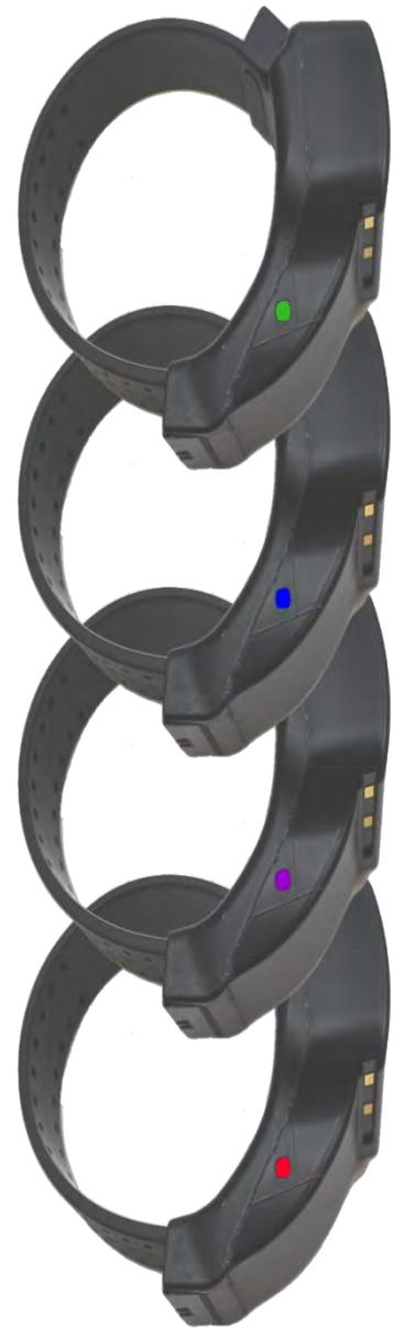
**Figure 39. LED Battery Notifications**
