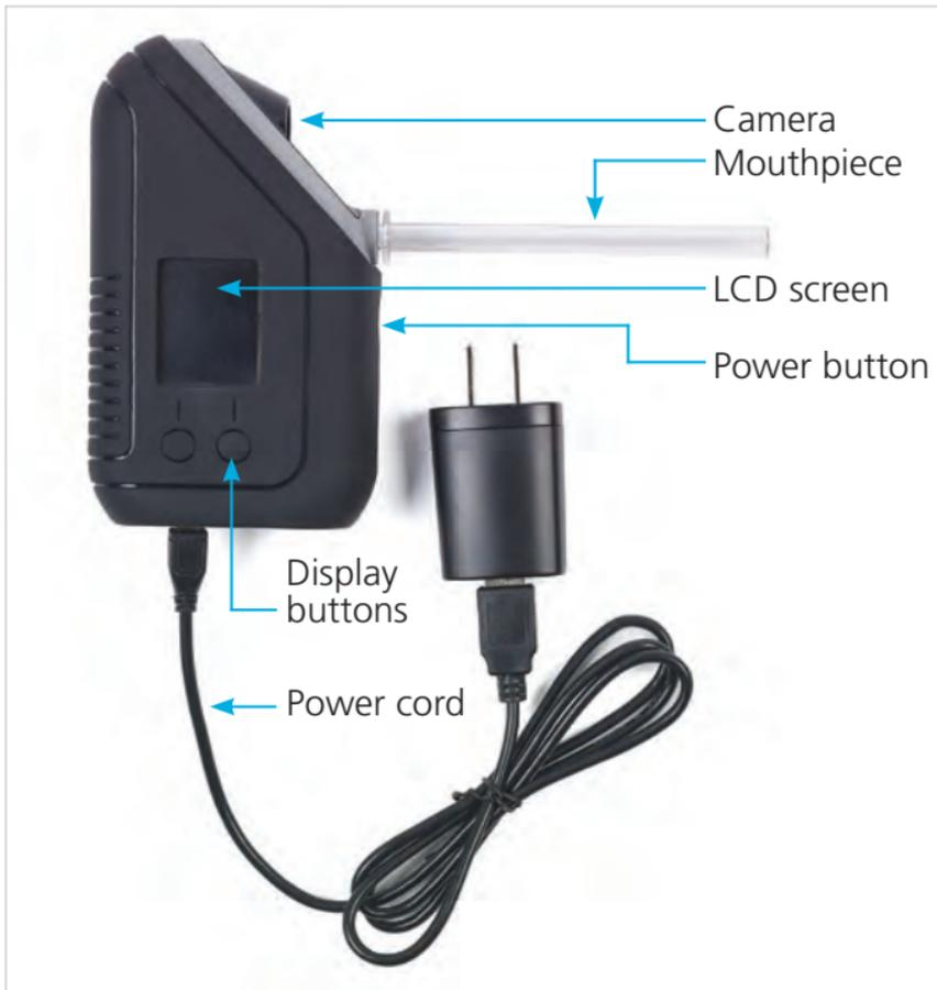
1. Press the power button once to turn on the BI SL3® device.
