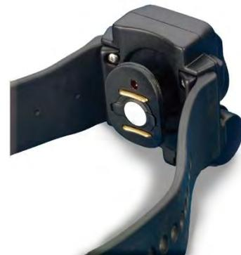
**Figure 66. Alcohol Detection Sensor**
