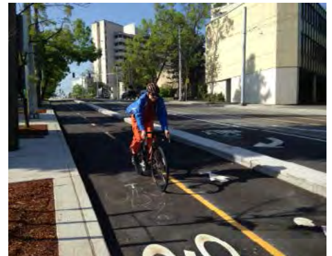
Two-way, on-street cycletrack
