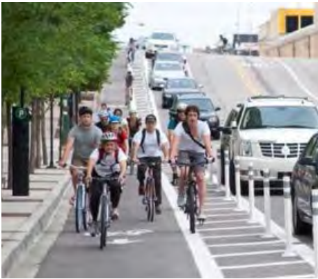
Buffered bike lane adjacent to vehicular lane
