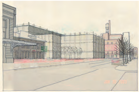
Examples of massing studies evaluating visual impact of zoning envelopes along Wynkoop Street frontage.
