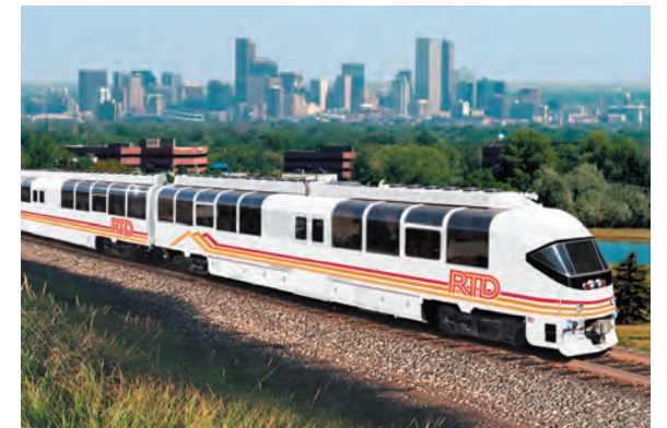
Diesel Multiple Unit (DMU).
