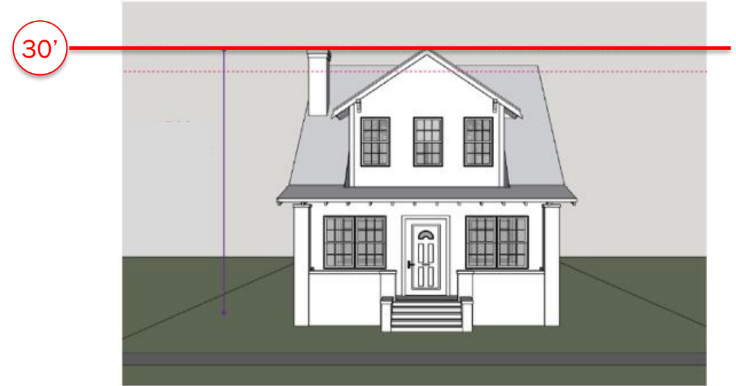
Pitched Roof: greater than 3/12 pitch
