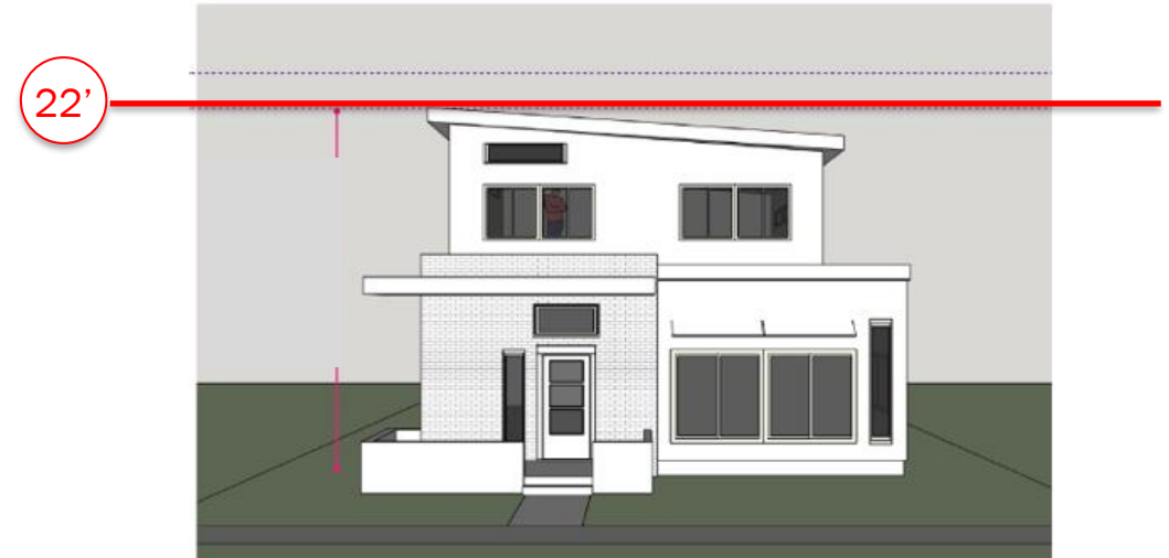
Low- Sloped Roof: 3/12 pitch or less
