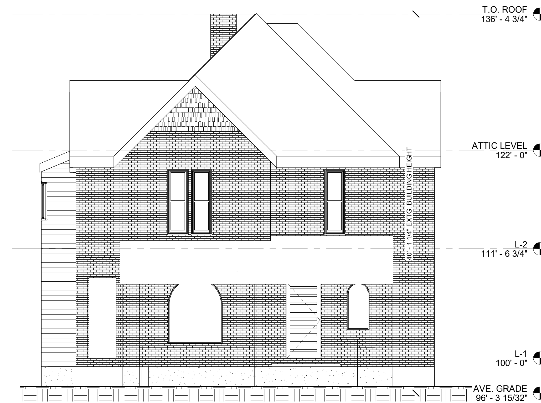
① EXTG. EAST ELEVATION 3/16" = 1'-0"
