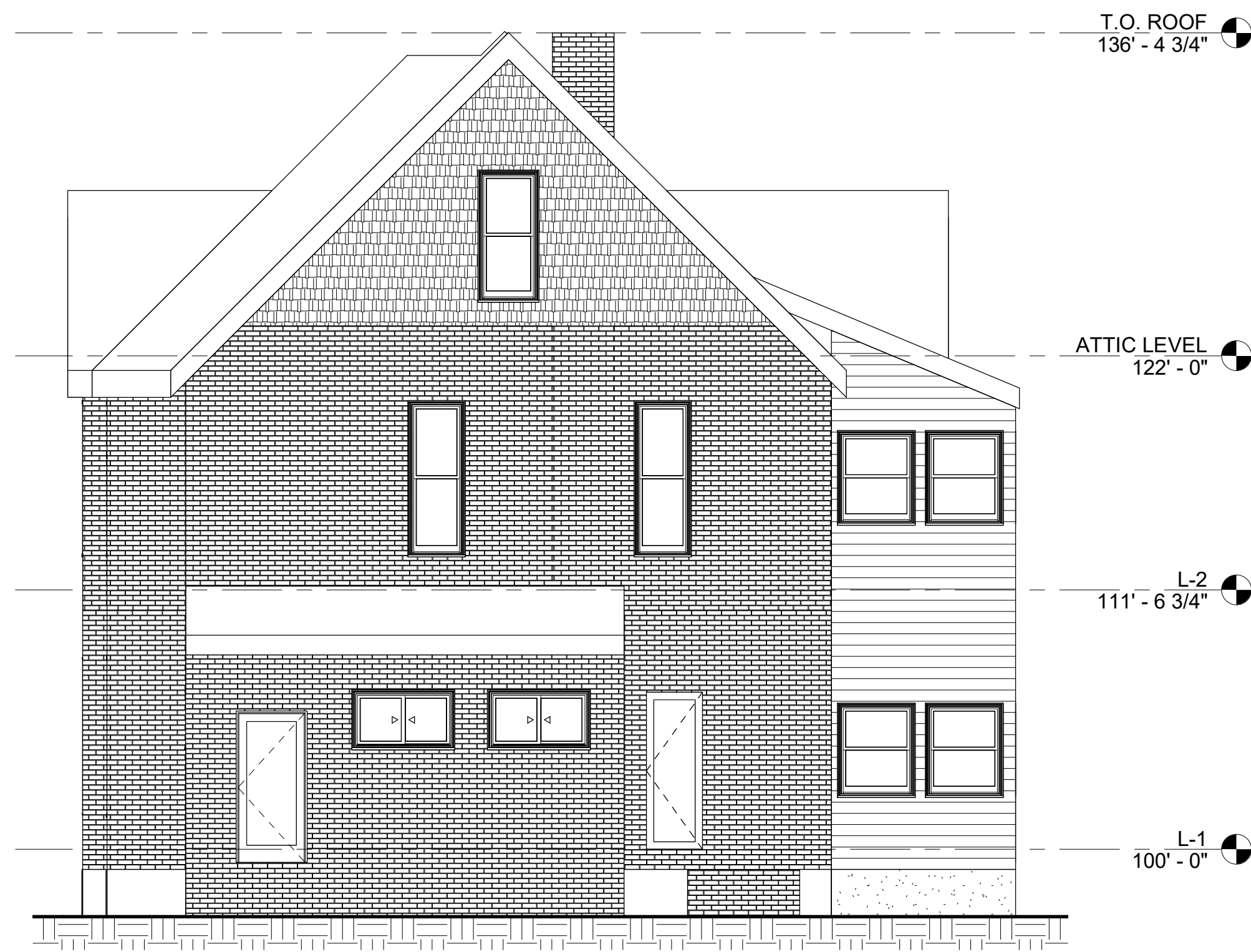
④ EXTG. WEST ELEVATION 3/16" = 1'-0"
