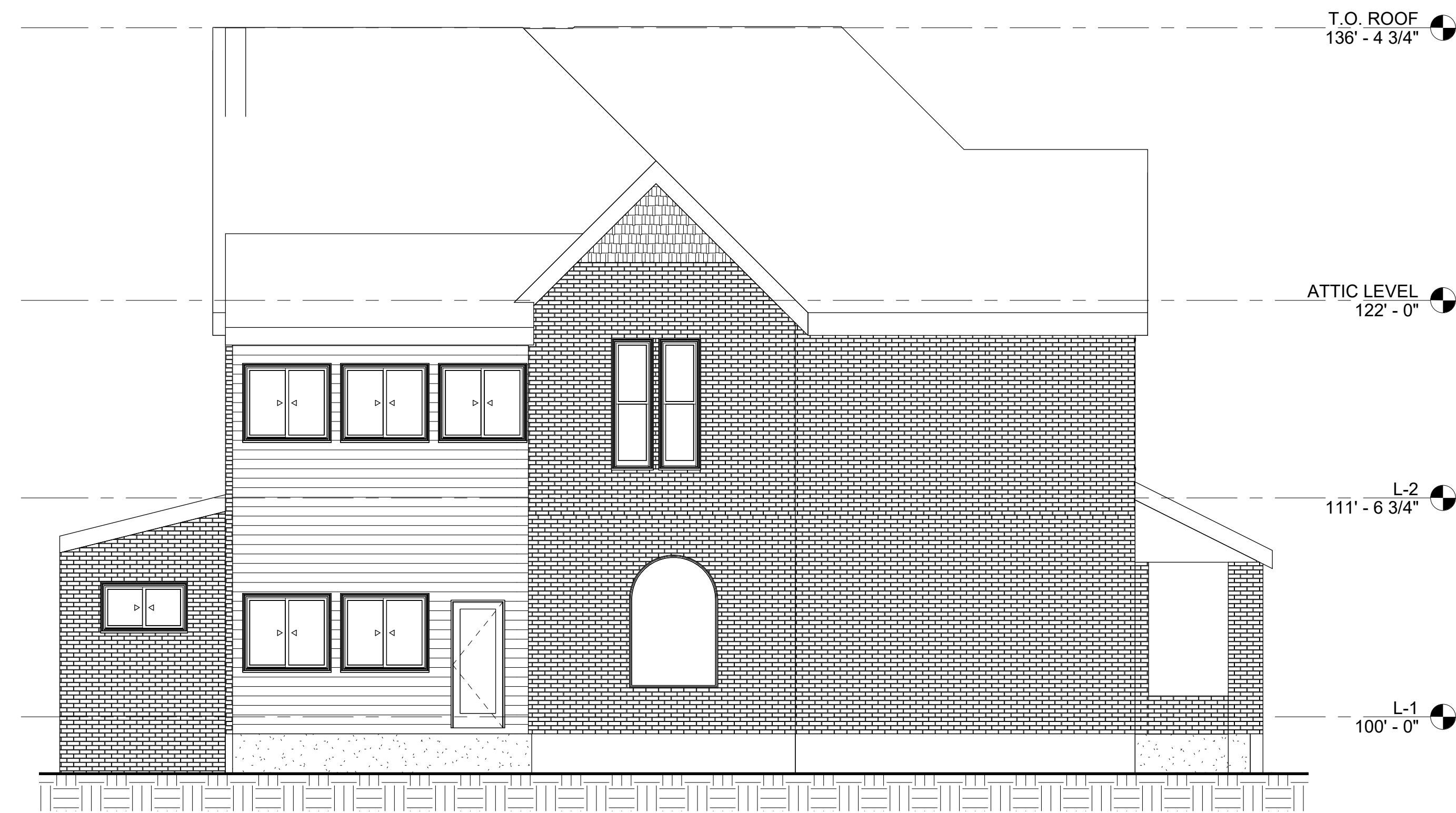
③ EXTG. SOUTH ELEVATION 3/16" = 1'-0"
