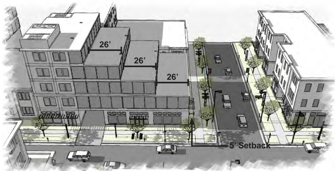
3rd Avenue Solar Access Bulk Plane: the bulk plane ensures that the sidewalk and amenity zone on the north side of 3rd Avenue are in sunlight for the whole year. This image shows the shadow at 12:00 noon on December 21st.
