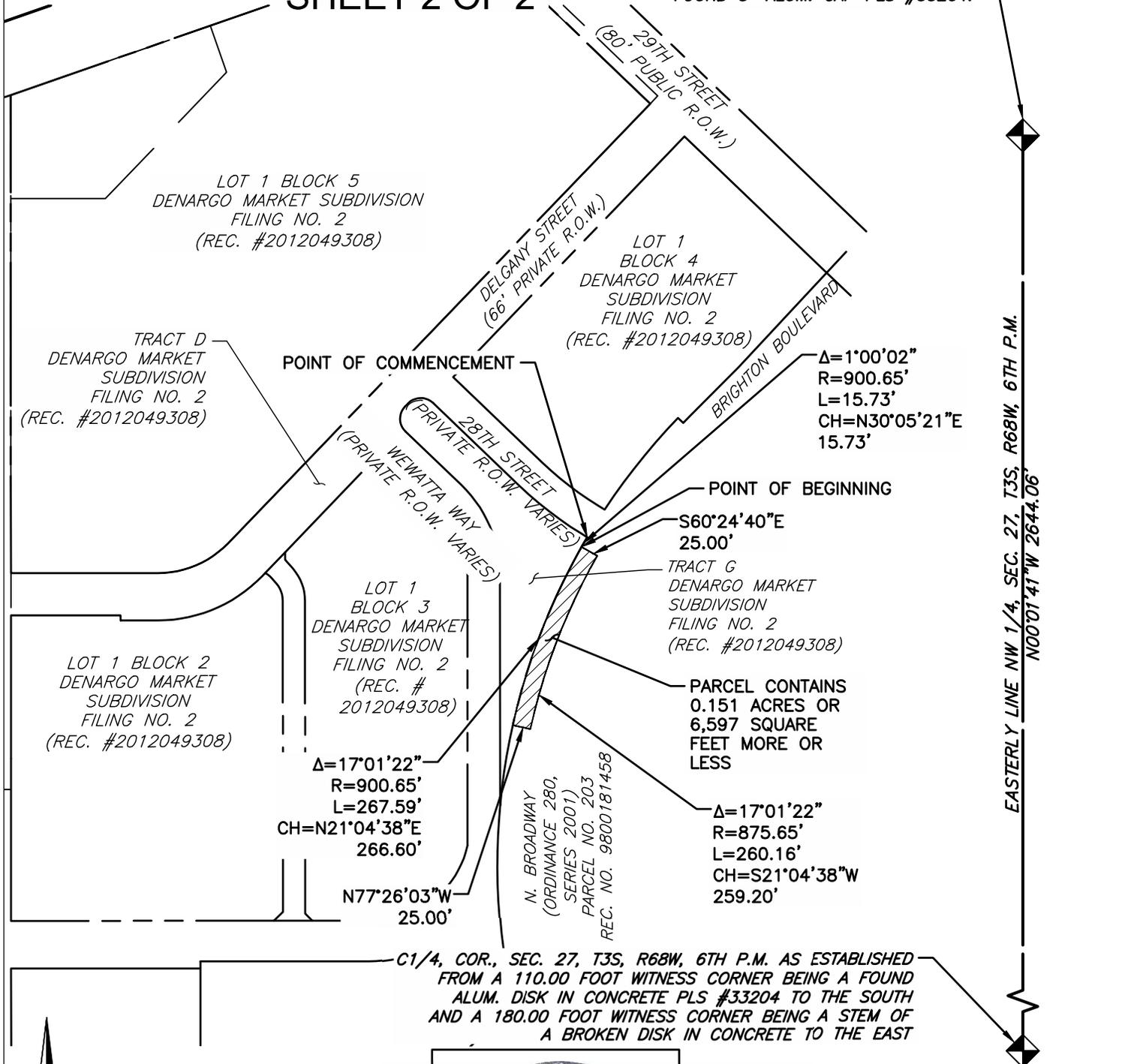
C1/4, COR., SEC. 27, T3S, R68W, 6TH P.M. AS ESTABLISHED FROM A 110.00 FOOT WITNESS CORNER BEING A FOUND ALUM. DISK IN CONCRETE PLS #33204 TO THE SOUTH AND A 180.00 FOOT WITNESS CORNER BEING A STEM OF A BROKEN DISK IN CONCRETE TO THE EAST
