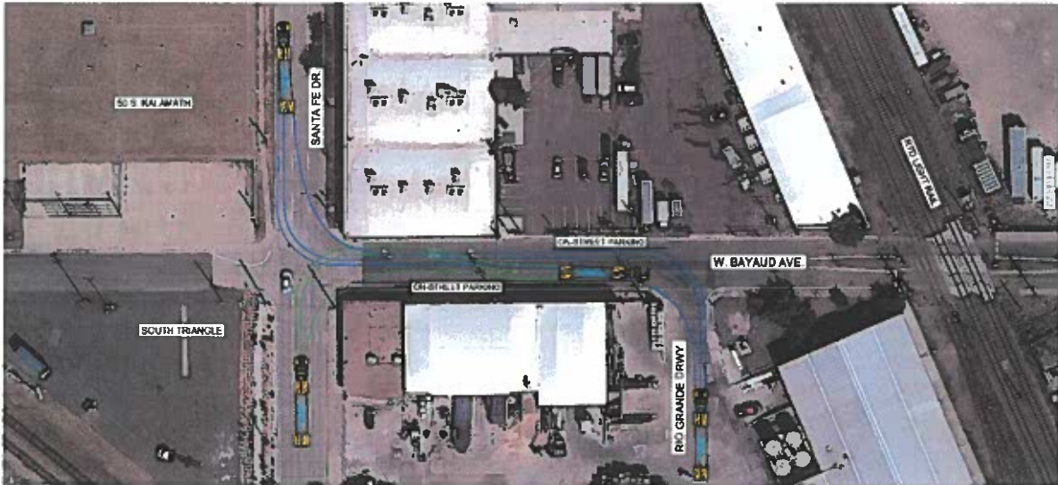
TRUCK TURNING MOVEMENTS USING BAYAUD ACCESS
