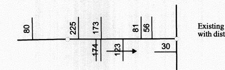
Existing Sanitary Service Lines with distance to downstream Manhole
