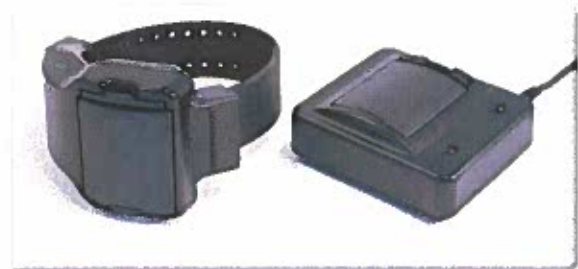
Figure 23. BI LOC8 and Beacon The beacon provides RF monitoring and also charges the LOC8 external battery.
