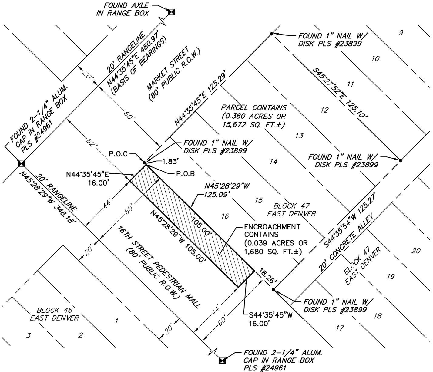
**BASIS OF BEARINGS:** BEARINGS ARE BASED ON THE 20' FOOT RANGE LINE IN MARKET STREET BEARING N44°35'45"E AND BEING MONUMENTED BY A FOUND 2-1/4" ALUMINUM CAP IN RANGE BOX PLS #24961 AT THE INTERSECTION OF MARKET STREET AND 16TH STREET AND A FOUND AXLE IN RANGE BOX AT THE INTERSECTION OF MARKET STREET AND 17TH STREET.
