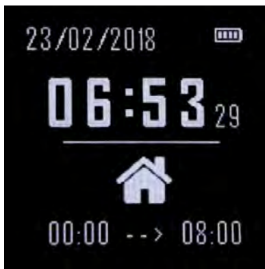
The ActiveWatch main screen displays the date, time battery status and current curfew.
