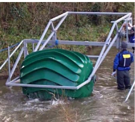
Hydro electric barrel.
