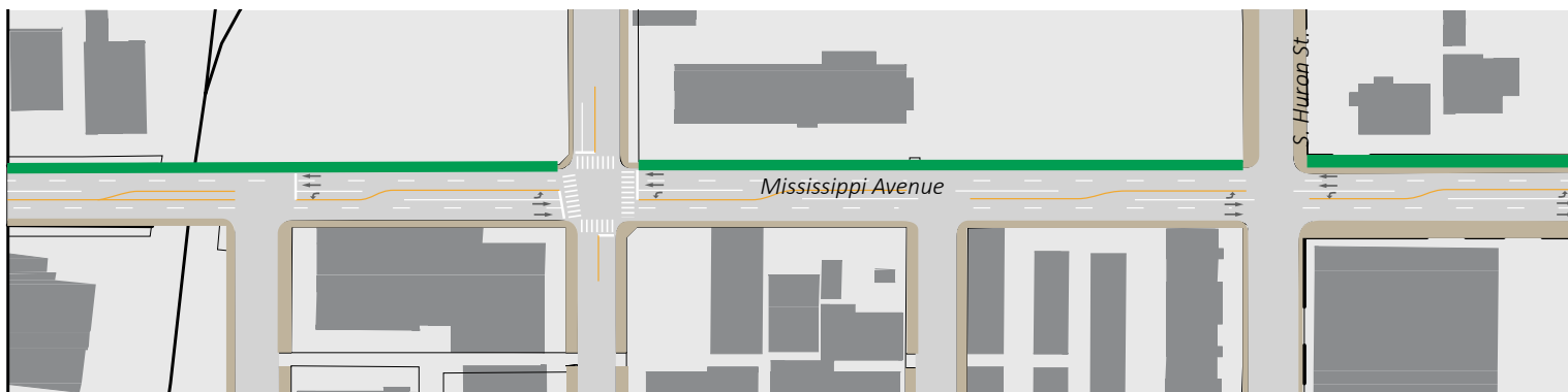
Mississippi Concept Diagram with Multi-Use Path on North Side of the street.
