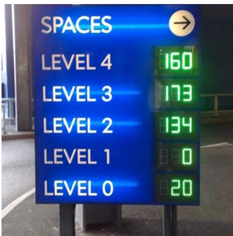
Parking Management Technology reduces air pollution by directing traffic to open spaces, reducing drive time
