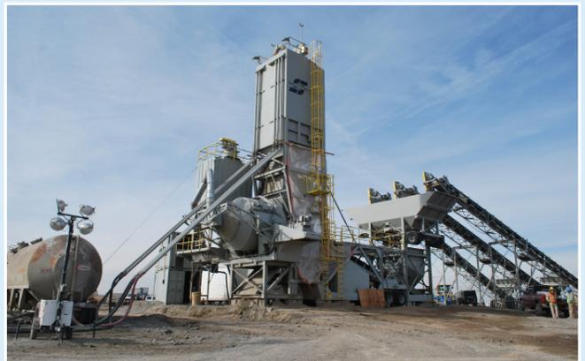
As of 2021, Flatiron's on-site batch plant carries six mix designs used extensively for our ongoing work at the airport.
