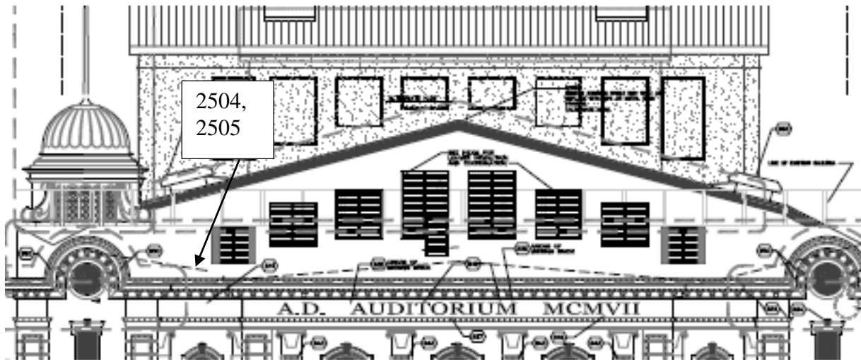
Figure 3. XRF reading locations, Ellie Caulkens rooftop, Galleria side.
