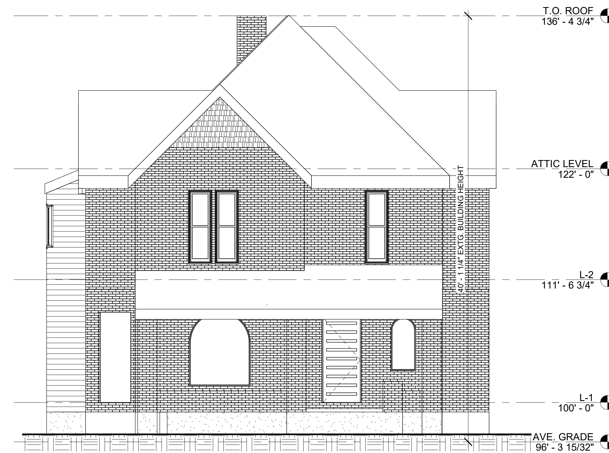
① EXTG. EAST ELEVATION 3/16" = 1'-0"
