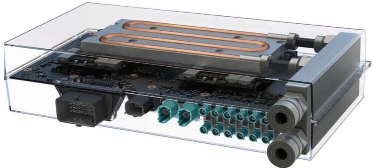
Nvidia Drive PX 2 : 250 watts 8 TFLOPS, 24 DL TOPS supercomputer Integrates LiDAR, Radar, Cameras
