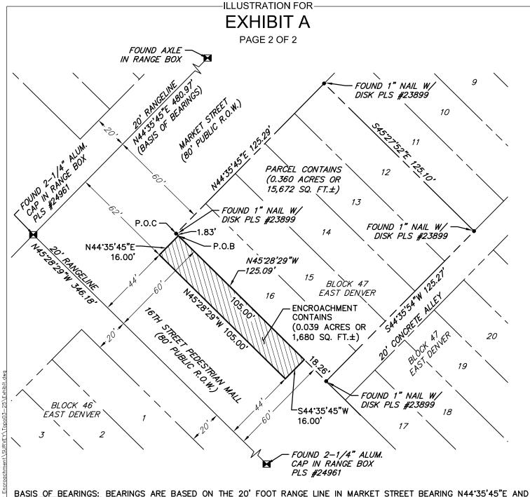
BASIS OF BEARINGS: BEARINGS ARE BASED ON THE 20' FOOT RANGE LINE IN MARKET STREET BEARING N44'35'45"E AND BEING MONUMENTED BY A FOUND 2-1/4" ALUMINUM CAP IN RANGE BOX PLS #24961 AT THE INTERSECTION OF MARKET STREET AND 16TH STREET AND A FOUND AXLE IN RANGE BOX AT THE INTERSECTION OF MARKET STREET AND 17TH STREET.
