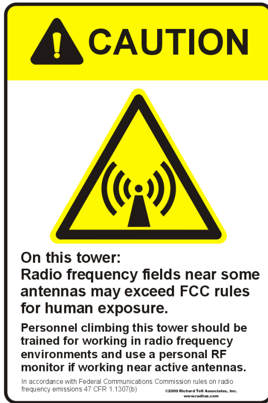
Figure 1 - Warning Sign to be Posted at Base of Tower (Available from Tescos, Holaday, Narda and other Sources)
