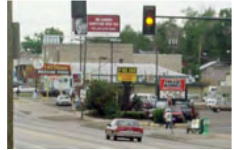
Too many access points (driveways) along commercial corridors can cause vehicle conflicts, reduce traffic flow and create an unfriendly pedestrian environment.
