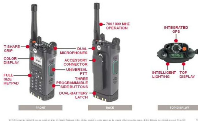
Figure 2-3: APX 6000 operational controls.
