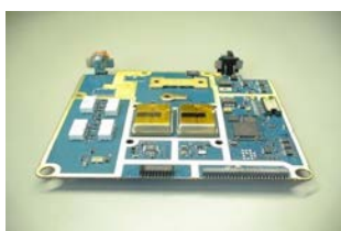
Figure 2-11: The APX has hard gold contacts molded into plastic to eliminate loose wires and parts
