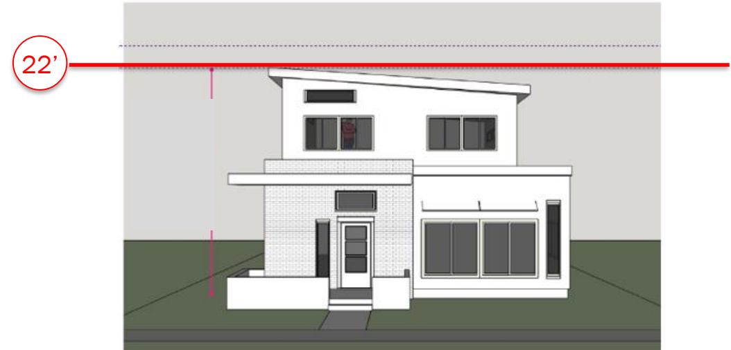
Low- Sloped Roof: 3/12 pitch or less
