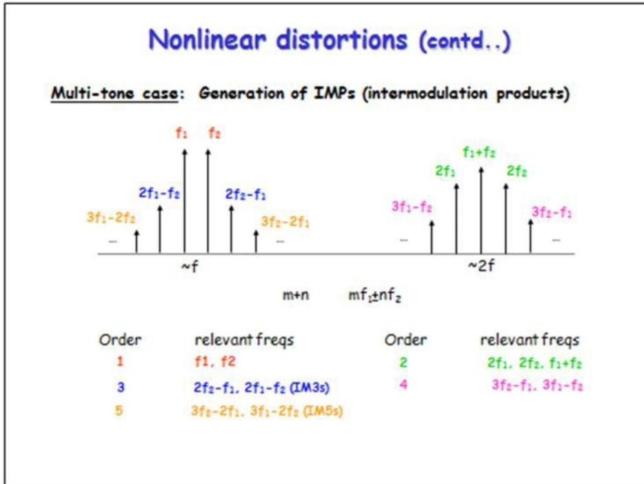
Not all of the mixing possibilities are significant in creating interference signals. Some fall “out-of-band” of the receiver and the higher order IM products are usually weaker in signal strength.
