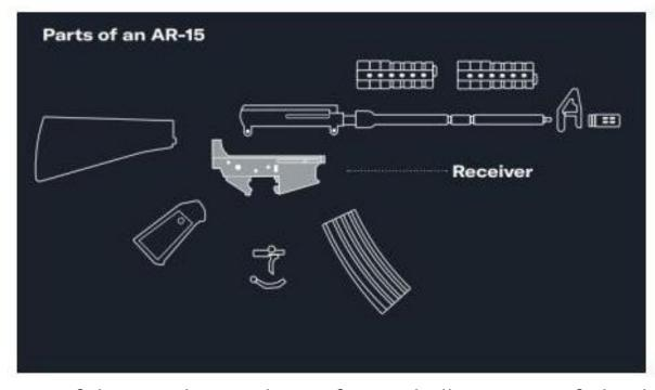
The frame or receiver brings together the trigger and other parts of the gun that are key to firing a bullet. Current federal law requires complete frames and receivers to have a serial number. Receivers that are not fully finished (80%ers) are not currently considered a firearm, not required to have a serial number, and do not require a background check to purchase.
