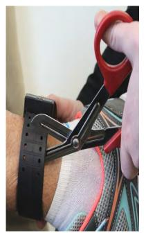
Figure 35. Cut-to-Fit Strap Design The LOC8 XT "cut to fit" strap ensures a secure and comfortable fit on the client's ankle, reducing the likelihood of a strap tamper.
