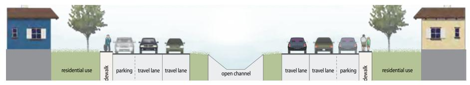
Montbello's existing residential collector streets feature two travel lanes in each direction and a parking lane, with the open drainage channel in the middle of the right-of-way.
