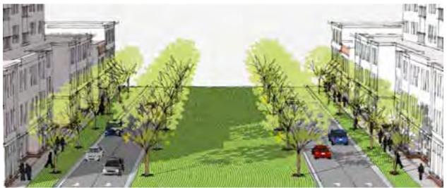
Telluride Street serves as a mixed-use arterial in the station area with four vehicular travel lanes and ample pedestrian zones but without on-street parking. The street has a wide parkway-like median with trees and a clear zone to accommodate the Phillips gas pipeline that travels from southwest to northeast through the station area. This cross section generally applies to Telluride north of First Creek and south of Blue Grama Draw.
