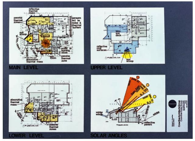
Figure 2: Details of Crowther's passive solar design at 401 Madison St. WH1504-2016-76
