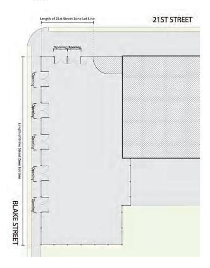
Figure 6.1. Required Unobstructed Openings for Fencing. Illustrative only.
