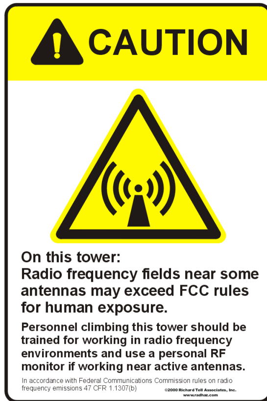
Figure 1 - Warning Sign to be Posted at Base of Tower (Available from Tessco, Holaday, Narda and other Sources)
