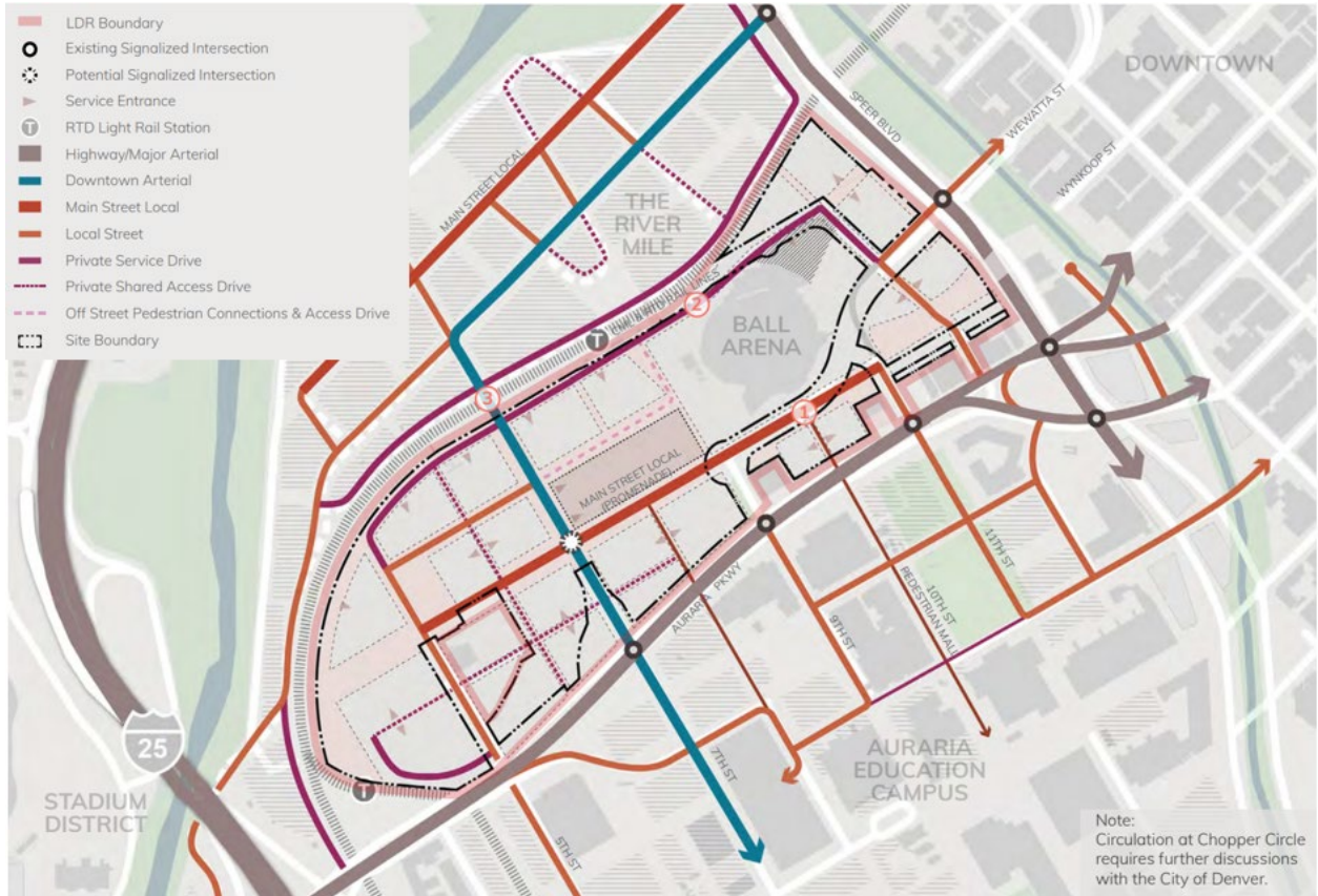
Figure 4 – Vehicular Circulation & Service Network
