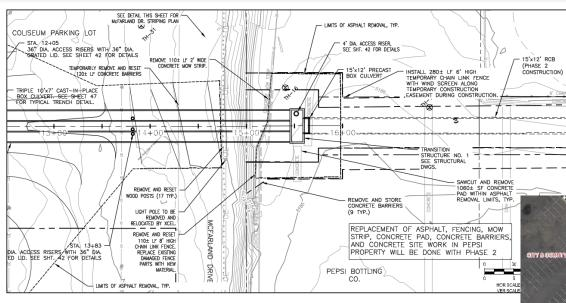
Construction of 15'x12' culvert and transition structure within Bottling Group property reduces their parking area during the period of construction
