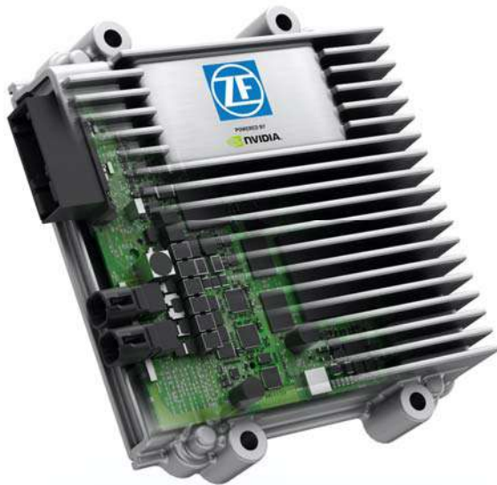
Nvidia/ZF Pro AI : 10 watts Computation = 150 MacBook Pros Integrates LiDAR, Radar, Cameras
