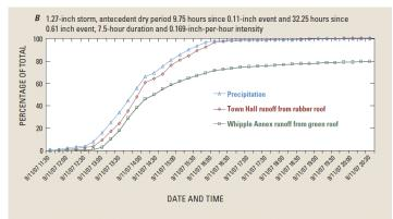
Figure 19. (A) Precipitation on and runoff from conventional rubber and green roofs in Ipswich, MA, for the storm of September 11, 2007, and (B) cumulative percentages of total precipitation and total runoff from the roofs for the same storm.
