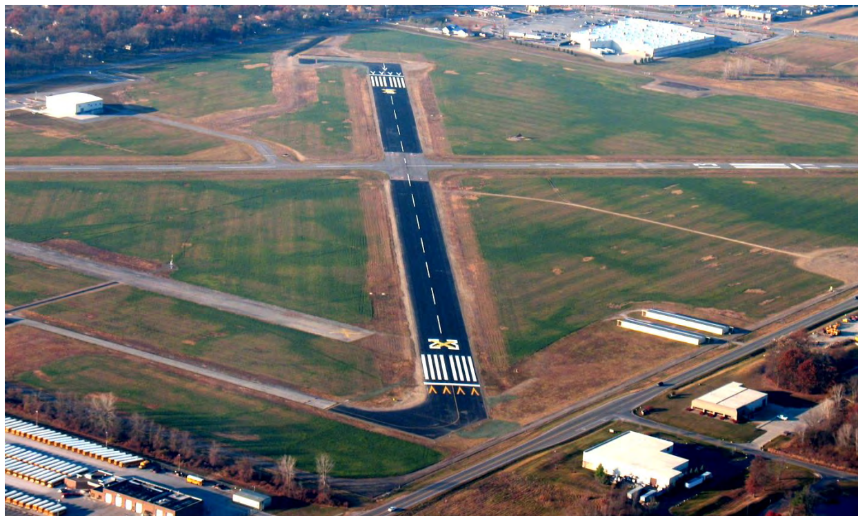
Figure 2-3. Markings for a Temporarily Closed Runway
