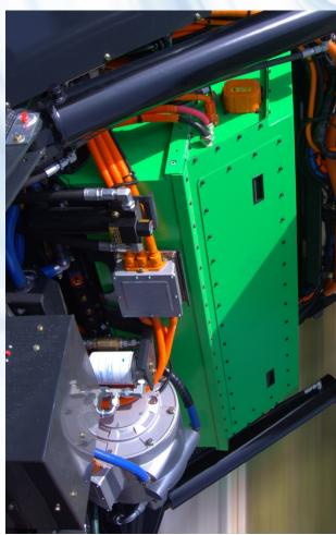
ALL ELECTRIC DRIVE SYSTEM Large Batteries will last for up to 11 hours of operation. With a 10 Year Life Span, the Batteries are designed to last and will not have to be replaced.
