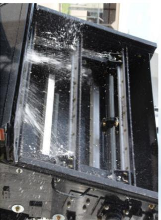
**HEAVY SWEEP PACKAGE** Elevator Type, Standard 11 Flight squeegee with replaceable corded rubber tips. Continuous molded rubber belts combine with standard Heavy Sweep Package make **Electric Global M4** the logical choice for sweeping heavy debris such as road millings, sand and gravel up to **3-tons per-minute**. That is one ton of sand every 20 seconds! Standard leaf gate system assists in picking up large debris, bottles, large branches and leaves.
