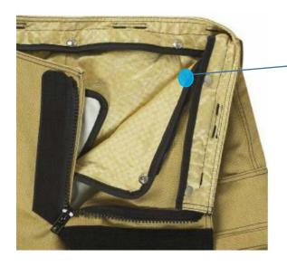
Inner flap to prevent zipper to touch the firefighter is attached to the liner with snaps. Each snap has a reinforcement to prevent from pulling out of liner
